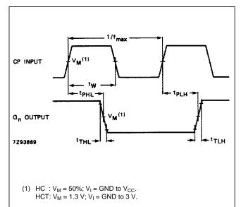
Fig.6 Waveforms showing the clock input (CP) pulse width, the CP input to output (Q<sub>n</sub>) propagation delays, the output transition times and the maximum clock pulse frequency.
