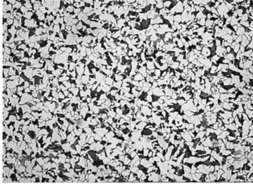
Figure 3.50 Microstructure at the core of PLC steel rebar
