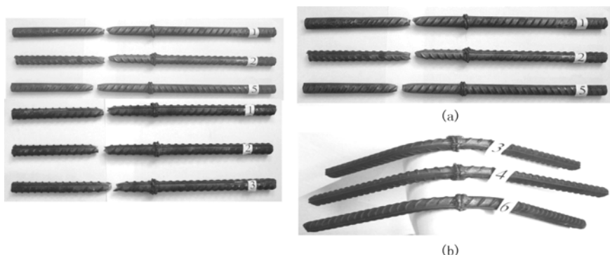
Figure 1.40 Weld specimens of ultra fine grain rebar steels
