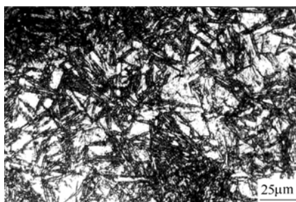
Figure 7.3 CFB morphology through treatment at isothermal temperature of 350°C
