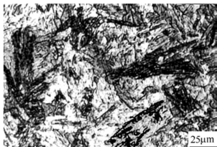
Figure 7.2 CFB morphology through treatment at isothermal temperature of 400°C
