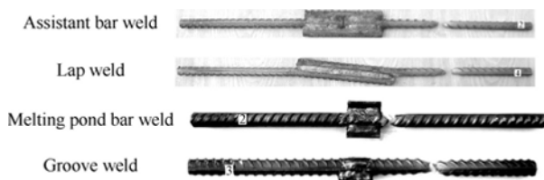
Figure 1.41 Tensile specimens of different welds of ultra fine grain steels
