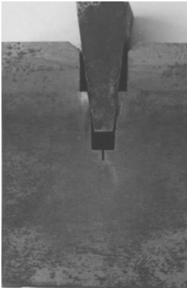
Figure 7.35 WOL constant displacement stress corrosion specimen for E-2 steel
