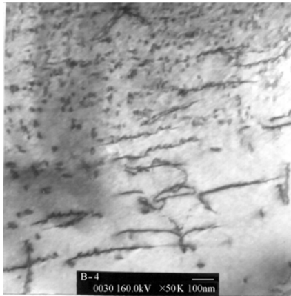
Figure 1.29 Secondary phase nanometer size precipitates of low alloy steel after rolling with deformation induced ferrite transformation
