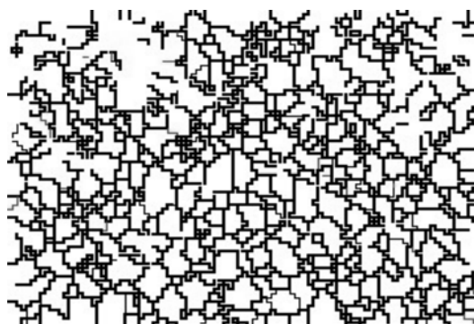
Figure 4.9 Microstructure graph of grain orientation for strip 1.9mm
