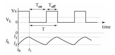
• For interval  $0 > t > t_1$ : diode is conducting:
