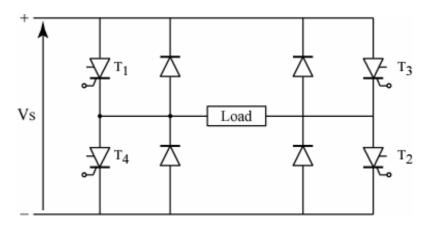
When T<sub>1</sub> is fired, we have class A chopper; when T<sub>3</sub> is fired, we also have class A chopper, but load voltage is reversed
