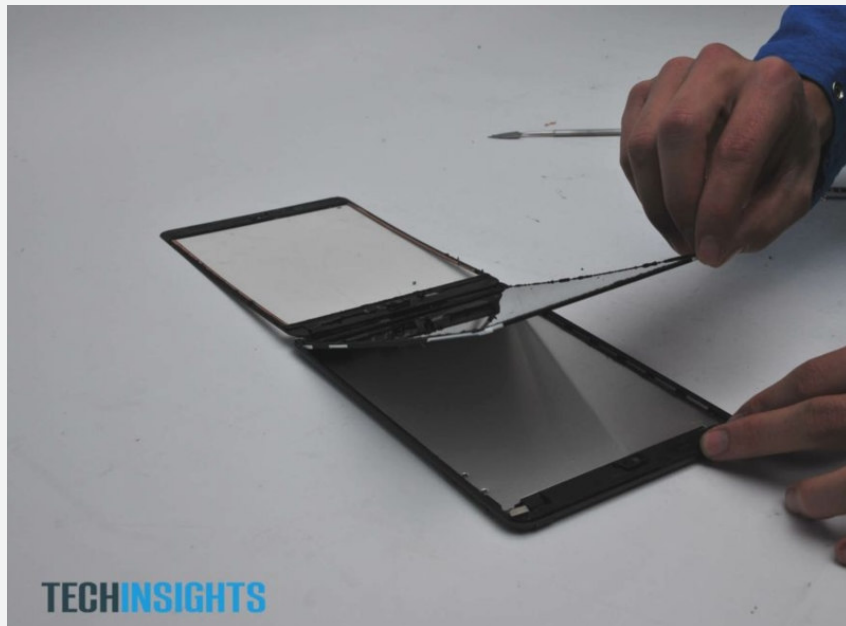
Separating the LCD display from the metal enclosure
