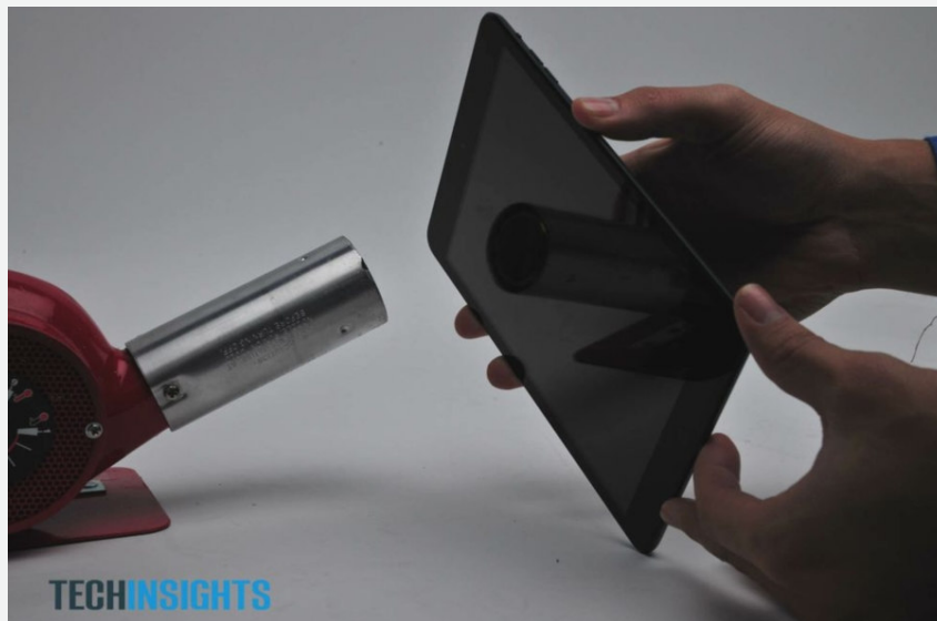
Using the heat gun to soften the adhesive around the touchscreen
