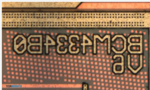
Inside the Murata module containing the Broadcom BCM4334.
