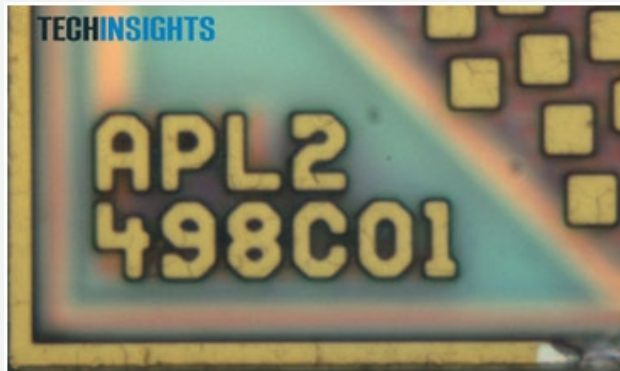
Die marking of the Apple A5 – 32-nm version.
