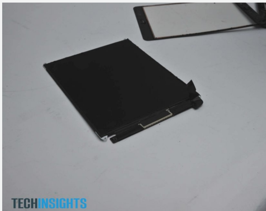
Another look at the LCD panel separate from the iPad Mini
