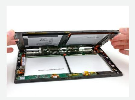
The iFixit folks found that they had to remove 17 pesky Torx screws to almost get the rear case off. The final step is to unhook the ribbon cable which tethers the battery to a connector on the motherboard.
