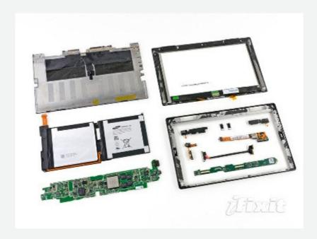
Our final photo displays the fully disassembled Surface. Ifixit, which focuses on DIY repair information, gives the Surface a 4 out of 10 repairability rating, mostly because of difficulties in removing the rear panel and keyboard connector, and because the LCD and glass are fused together, which means increased repair costs. Read iFixit's complete teardown here.
