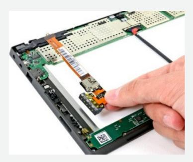
This shot shows the large orange ribbon cable leading to the SUrface's magnetic charging port. A microSDXC card slot underneath the kickstand is also attached to the ribbon cable
